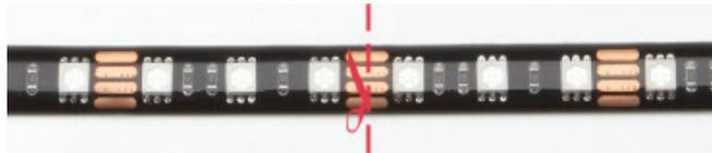
*Note: Do not cut strip while connected to power source. Do not let end of cut strip touch frame of bike. Wrap the cut end of the strip with a small piece of electrical tape or better yet seal the cut end with Silicone Sealant. Silicone Sealant is included with this Kit. Cut ends of strips that are not covered will cause a Negative Short causing the Lights to come ON very DIM and burn the circuits of the Remote Control Box. To prevent this, make sure you seal cut strips!*
